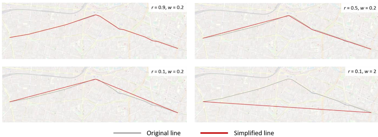
Figure 5.10: Impact of different r values and weight factors on the simplification of a polyline with data-based calculation of the \epsilon value. Map data from OpenStreetMap.
