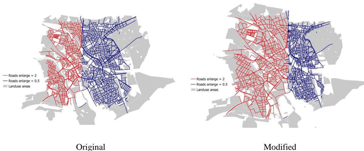
Figure 5.15: Geometric deformation of an entire road network and land use areas in a specified region using PUSH.
