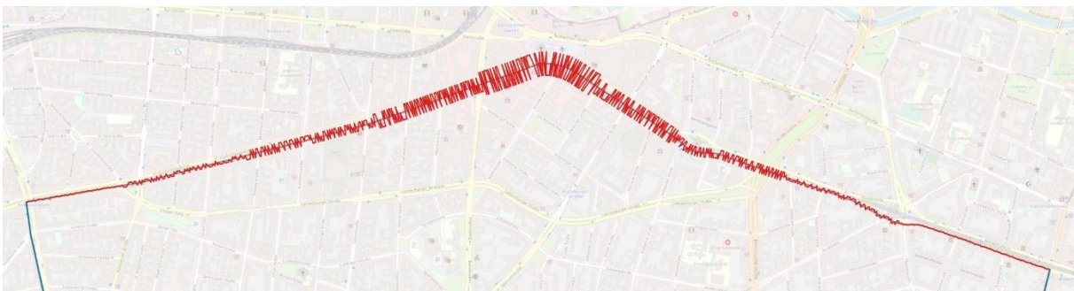
Figure 5.8: Visualization using data-based calculation of both factors d (distance from line) and np (number of points), polyline segmentation with seg = 20 meters. Map data from OpenStreetMap.
