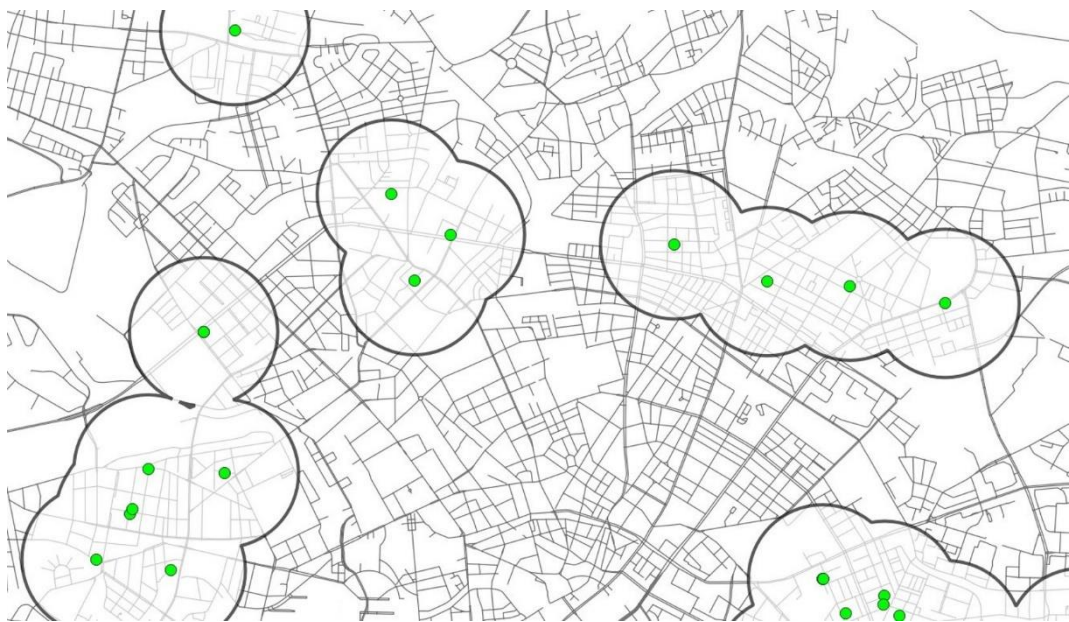
Figure 5.16: Definition of risk zones by dissolving buffer areas around locations of negative impact.
