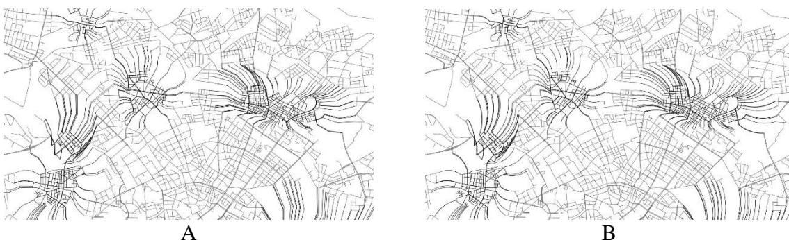
Figure 5.17: Application of the multi-scale deformation approach to several risk areas of different shapes and different risk level. A = knee connector, B = curve connector. Risk area deformation in both maps corresponds to the risk areas as defined in Figure 5.16.
