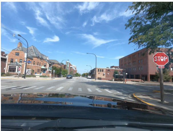
(e) All-way stop controlled intersection (Four-leg inter.).
