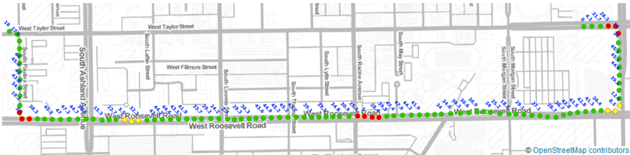
Figure 4.4.: Stopping (red) and deceleration (yellow) episodes detected in one trip (from east to west). The numbers in blue indicate the vehicle's speed in kmh.
