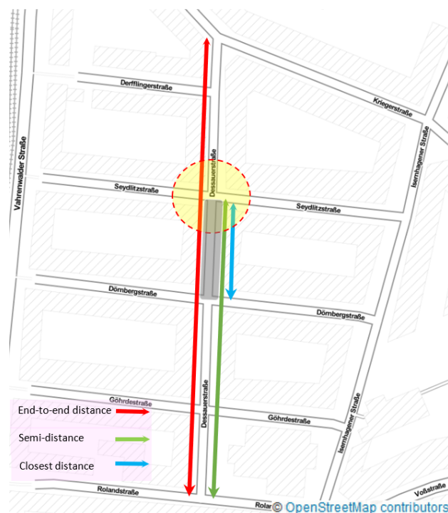
Figure 4.6.: Illustration of the distance-related features (end-to-end distance, semi-distance and closest distance) of the static method that represent the north-south intersection arm (indicated in grey color) of a four-way intersection (in yellow).
